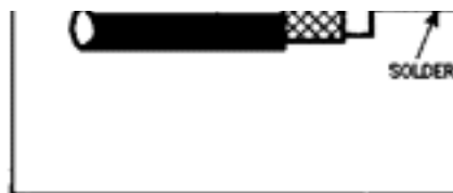
Figure 5. Each joint between the elements, and the joint at the feedpoint, is made like this.
